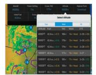
Aircraft performance tables in Garmin Pilot make it easy to input figures for such calculations as power setting and fuel/distance profiles. Calculations take into account such factors as outside air temperature, altitude and more.
