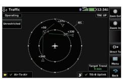
With ADS-B "In" from a compatible receiver (sold separately), the aera 660 and aera 760 can display traffic enhanced with Garmin TargetTrend™ technology, which shows target trajectories relative to your aircraft.
