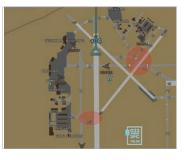
Optional SafeTaxi diagrams with georeferencing capability help you navigate on unfamiliar airports. With an optional GDL 52 series receiver, TerminalTraffic technology displays ADS-B equipped surface targets right on these diagrams.
