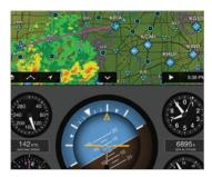
In addition to ADS-B weather and traffic, you can also view 3-D synthetic vision and backup attitude reference¹ provided by the GDL® 39 3D portable ADS-B receiver.
