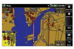
For low-flying helicopters and patrol aircraft, Garmin WireAware™ wire-strike avoidance technology offers added protection against powerline incidents.
