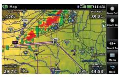
With ADS-B "In" data from compatible devices (sold separately), the aera 660 and aera 760 can display subscription-free U.S. weather and traffic, overlaid on the moving map.
