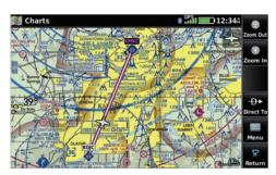
IFR Enroute and VFR Sectional charts for the U.S. feature georeferencing capability — with an overlaid aircraft symbol indicating your current position.
