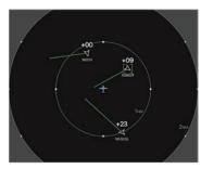
With an optional GDL 52 ADS-B receiver, Garmin Pilot can display subscription-free weather and datalink traffic. Traffic displays with our patented TargetTrend technology that shows traffic trajectories relative to your aircraft.
