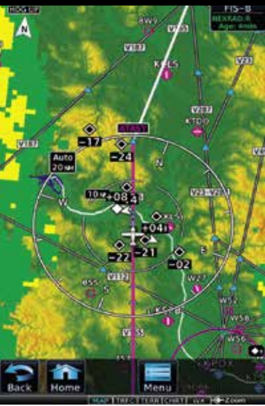
Integration of traffic and weather on a Garmin moving-map display provides critical situational awareness of potential flight-path conflicts.
