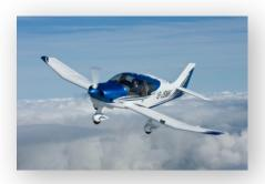
Contrary to myth, modern Robin aircraft do not need hangarage. The upper surface of the wing is covered in a 0.6 mm laminar, ensuring a durable and waterproof surface.
